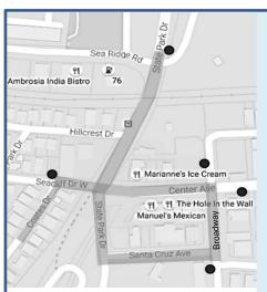
Utilities to be undergrounded are located within the shaded area with conduits connecting to recently installed utility poles shown as the dark circles at the edge of the project area. Utility poles in the alley between Center and Santa Cruz Avenues will also be removed.
